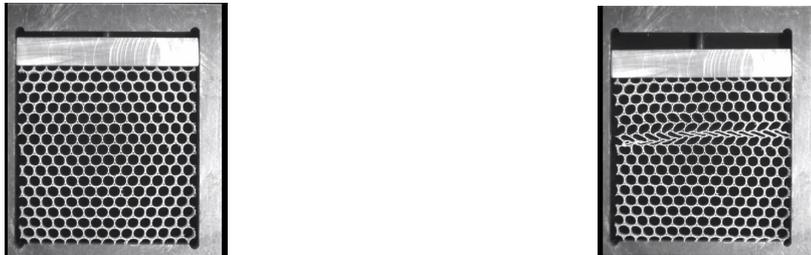
FIGURE 1. Compression of a circular honeycomb in a staggered stack
