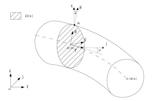
Figure 1.— Geometric characteristics of the pipe
