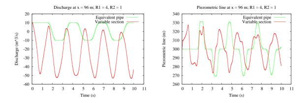
Figure 8.— Discharge (left) and piezometric line (right) for  $R_1 = 4 m$
