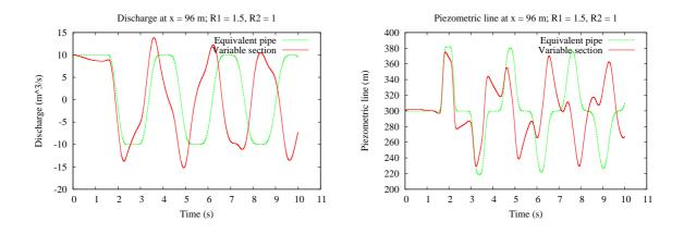
Figure 7.— Discharge (left) and piezometric line (right) for  $R_1 = 1.5 m$
