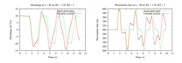
Figure 6.— Discharge (left) and piezometric line (right) for  $R_1 = 1.25 m$
